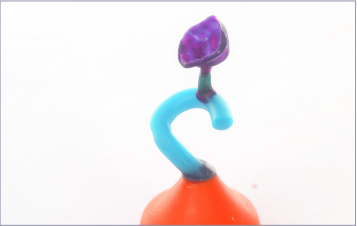
wax pattern attached to sprue ready for investing
